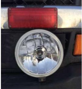
As a solution, effective immediately, BCEHS is removing the lens covers on all ambulance driving lamps to improve the forward-facing lighting in pattern and range. More on this, below.
